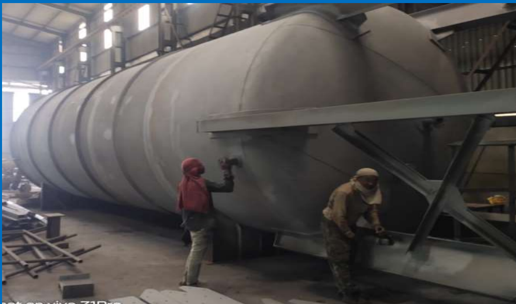
100 KL SHELL FABRICATION
